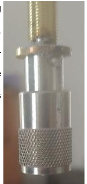
Figure 2: Closeup of the brass locknut soldered to the rear of the coax plug and also to the threaded lamp pipe.
