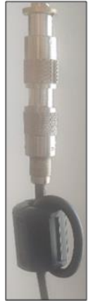
Figure 4: A snap-on ferrite toroid is attached to act as a common-mode choke
